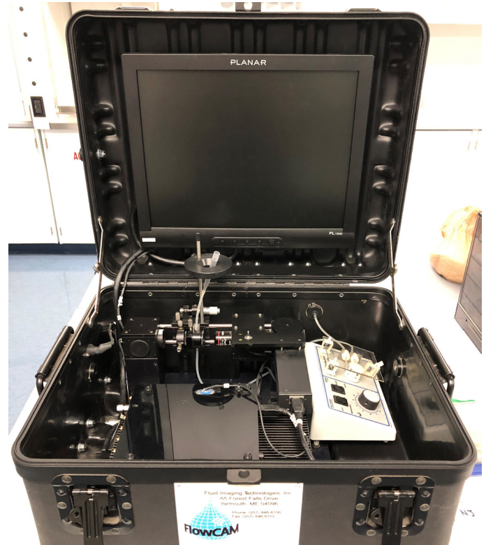
ABOVE: Hydro International's portable FlowCam, purchased in 2008. This model can be easily transported for field research. Fluid Imaging's improved and updated model, the FlowCam 5000, provides a similarly lightweight and portable solution for field studies.
